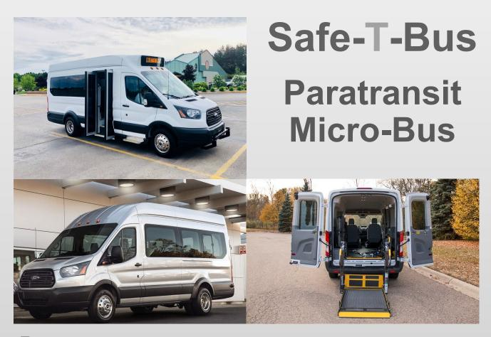
Safe **T**Bus has unparalleled versatility allowing endless possibilities for the transport of both ambulatory and non-ambulatory riders. Built on the popular Ford Transit chassis, Safe **T**Bus is the most serviceable and cost effective vehicle for your budget. With combinations from 3 lengths, 3 roof heights, and 2 engine choices you can customize your Transit to fit your unique needs. Available in gas, propane, CNG, Full Electric.
