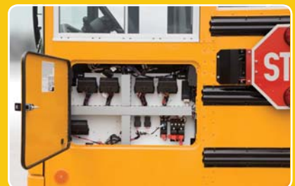
Redesigned exterior electrical access compartment for easier service.
