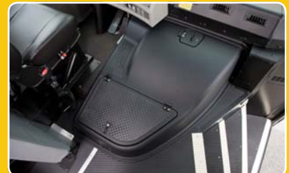
Redesigned engine access provides wider aisle for easier passenger loading and serviceability.
